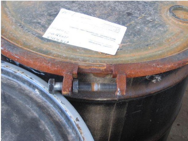
Notice bolt not tightened completely.
