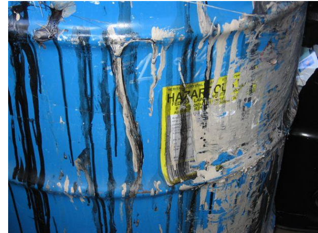
Non-DOT approved drum Hazardous Waste Label is covered with waste. Shipping labels must be completely visible and legible.
