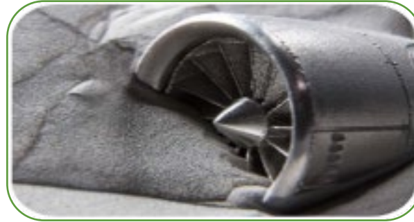
Metal powders used in Direct Metal Laser Melting, Powder Bed Fusion
