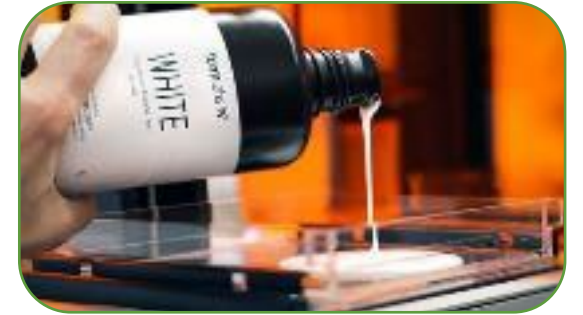
Liquid resins used in Stereolithography, Vat Polymerization
