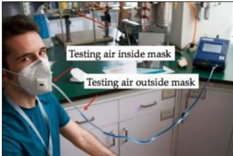
Figure: a typical respirator fit test using a PortaCount
