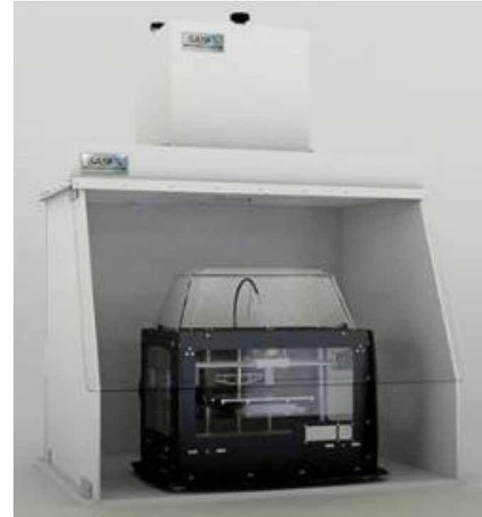
Example of a ventilated enclosure that contains and captures 3D printer emissions. Photo by NIOSH.
